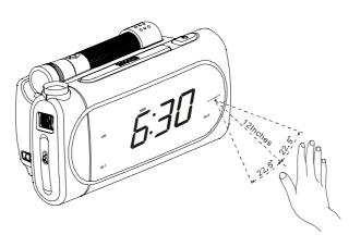
The Touchless Snooze Control works by detecting body heat. For best results your hand should be within <u>24 inches</u> of the front panel.
